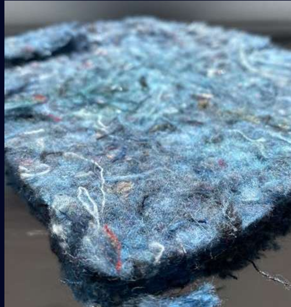
Generic acoustic insulation material removed from the inside of a domestic washing machine.
