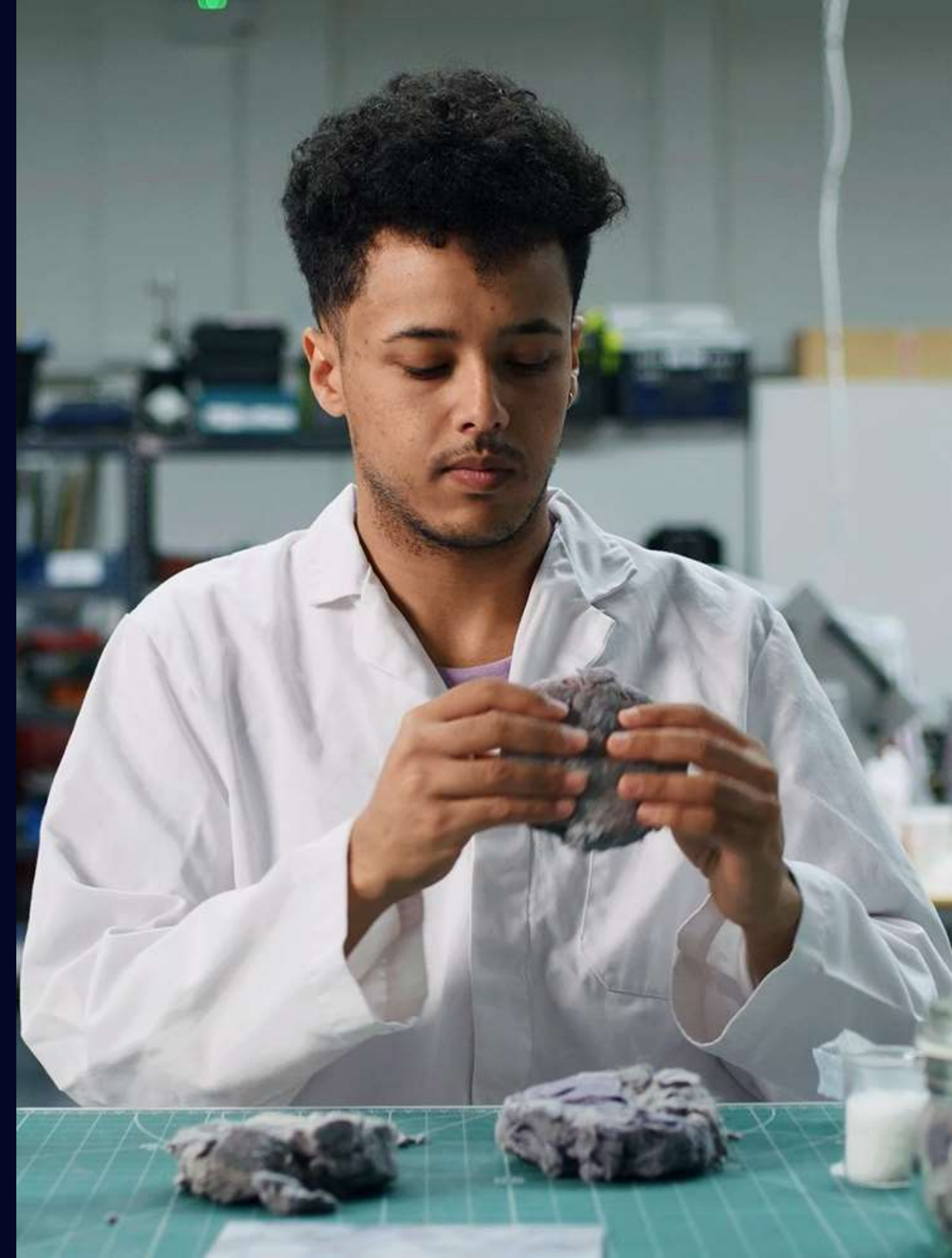
Generic acoustic insulation material removed from the inside of a domestic washing machine.
