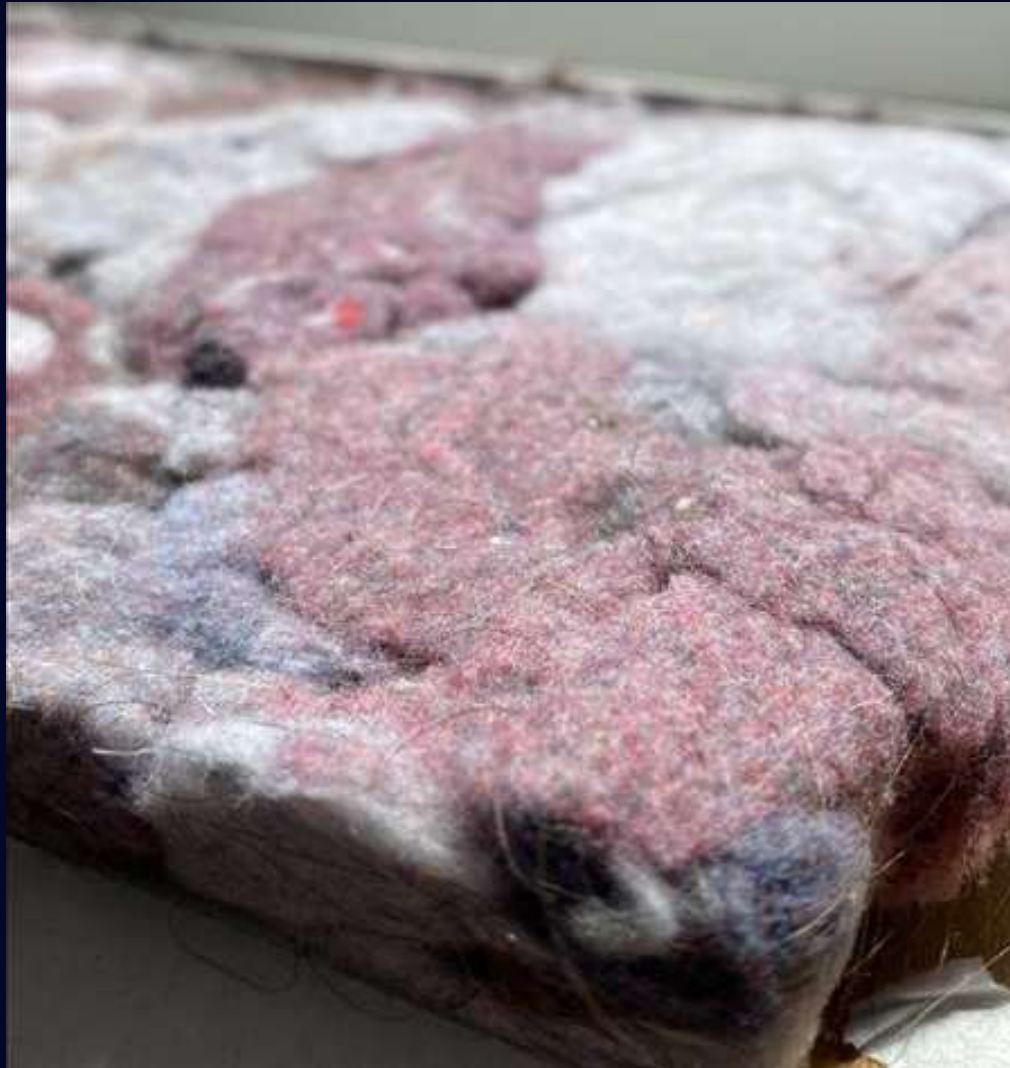
Matter proprietary insulation material based on recovered laundry effluent.
